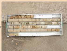
Geotechnical core from drilling in Walvis Bay harbour
