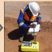
Geotechnical testing to validate compaction quality of road layers
