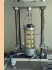
Geotechnical testing of soil samples to determine strength of foundation soils
