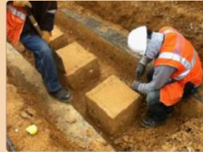
Collection of soil samples to determine strength of foundation soils
